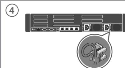
4. Loop and secure the power cable in the retention clip.
