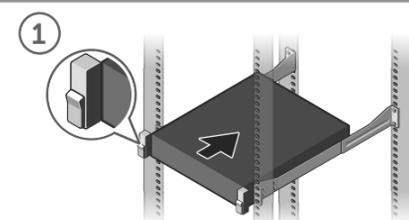
1. Install the system into a rack.
